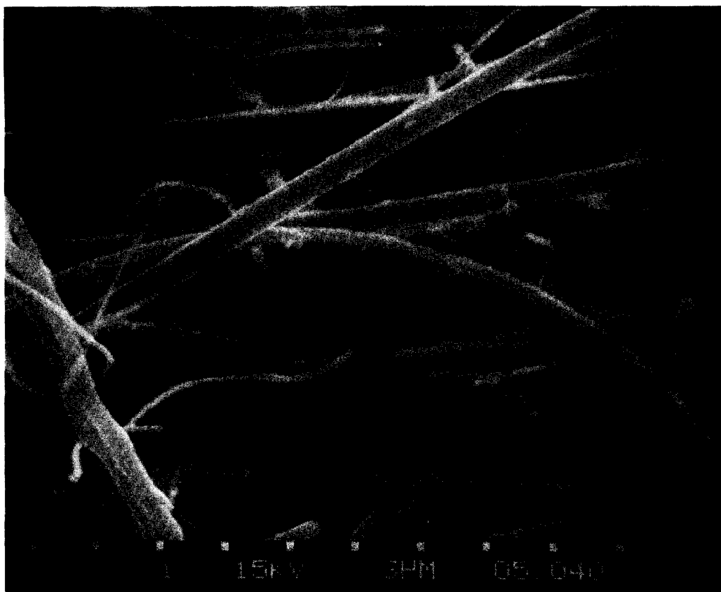
FIG. 7. Scanning electron micrograph of the glass fibers of a Whatman glass fiber filter.
