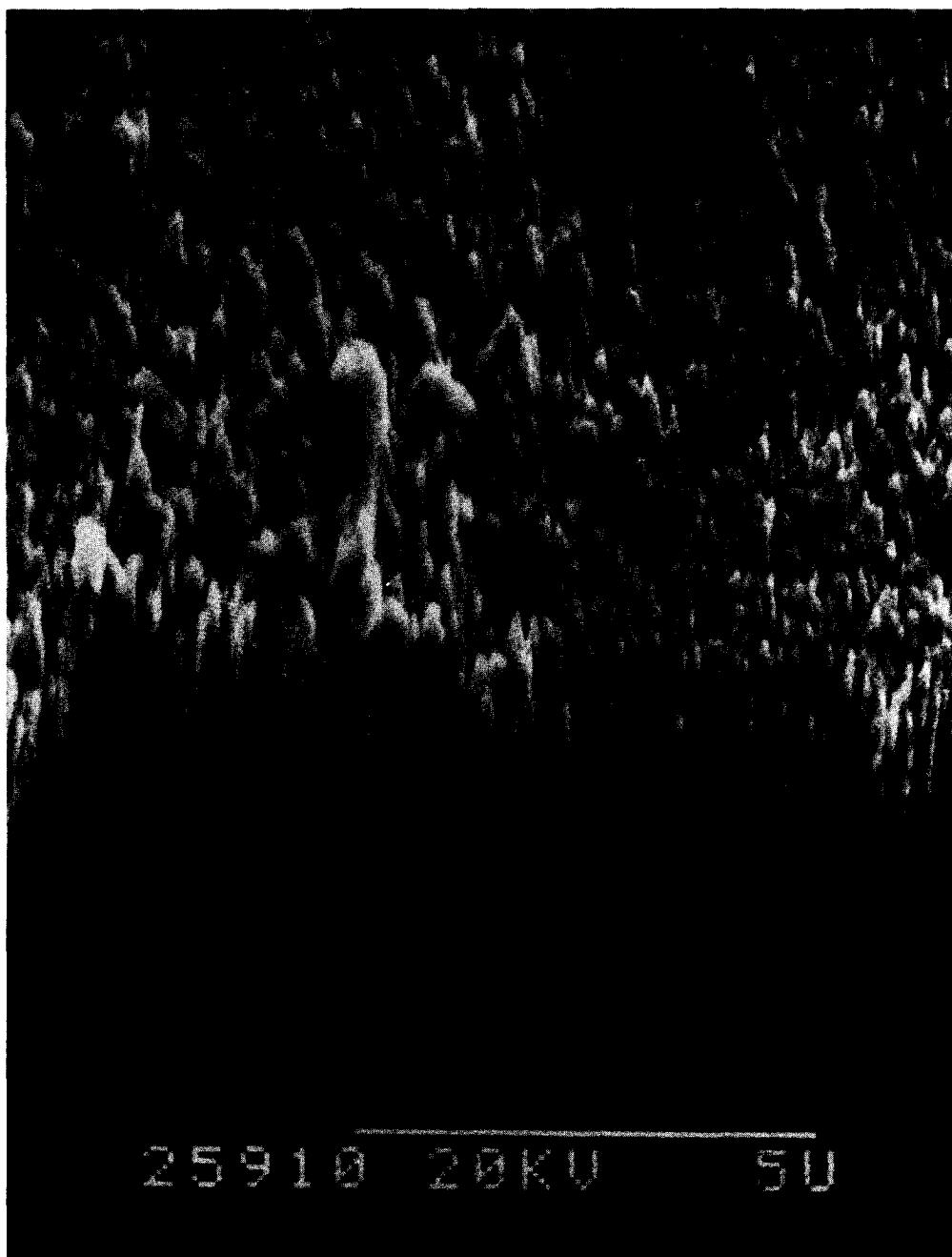
FIG. 10. Scanning electron micrograph of the anodic oxide structure of the type A catalysts.
